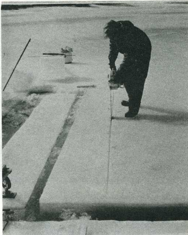
Figure 4. Preparing the ice for in-place cantilever beam tests. Also note at the left bottom of the figure the free end of the beam with the breaker device set up for a push-down test.
